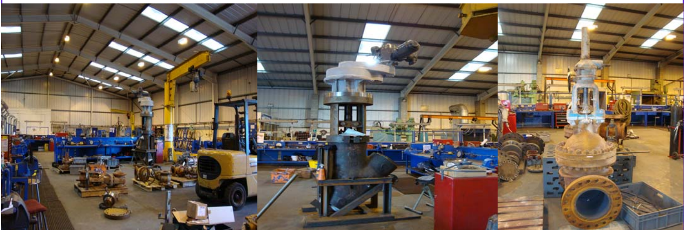
Foreground: RUSAL Aughinish Alumina Refinery Gate Valves being refurbished in the workshop.
